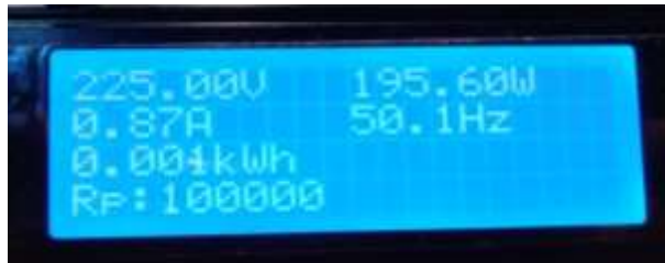
Figure 18. LCD Display Using Two 100 Watt Lights
