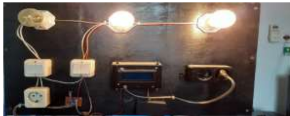
Figure 17. Power Testing Using Two 100 Watt Lights
