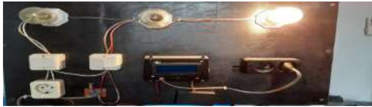
Figure 15. Power Testing Using One 100 Watt Lamp
