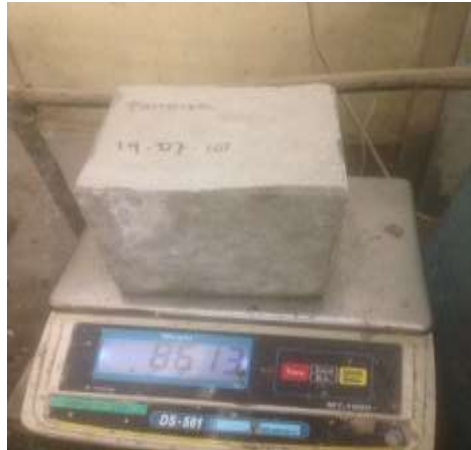
Figure 1. The strong test object is weighed before the compressive strength
