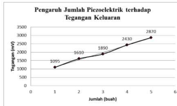
Figure 9. the effect of the number of piezoelectrics on the output voltage
