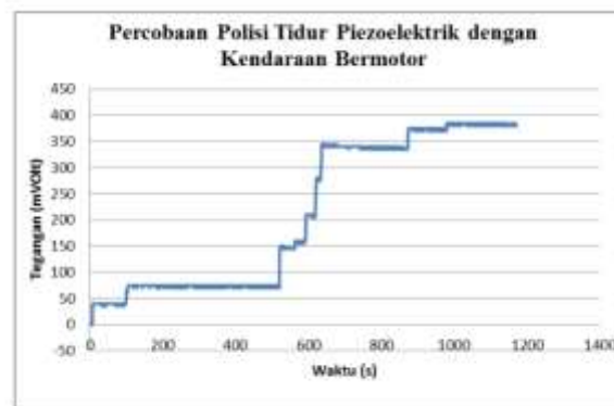
Figure 10. Test results of piezoelectric speed bumps with motor vehicles
