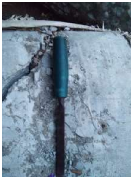
Figure 21. Chisels are used to make sound holes in the Keteng-keteng
