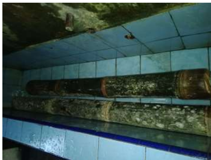
Figure 14. Soaking the bamboo material from Keteng-keteng Telu Ngawan
