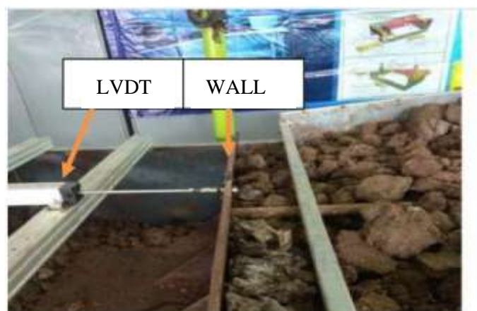
Figure 1. LVDT Conect to the Wall
