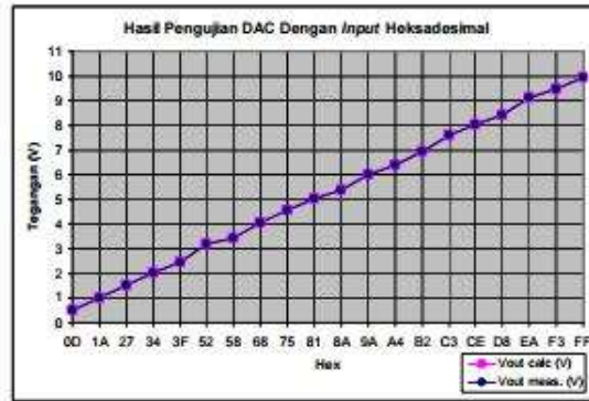
Figure 6. Output Voltage Graph Using Hexadecimal Input
