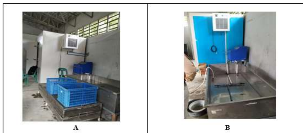
Figure 2. An ozone generator device, an ozone dissolution tank with micro bubble technology and a cold storage filled with ozone are used at the Chili Farming Center, Lubuk Cuik Village, Lima Puluh Subdistrict, Batu Bara Regency, North Sumatra.
