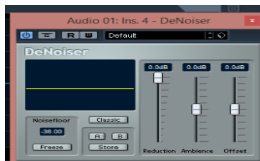
Figure 16. Plug-in De Noiser setting to reduce Noise
