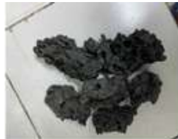
Figure 7. Biofilter media for plastic coral type manufacturer
