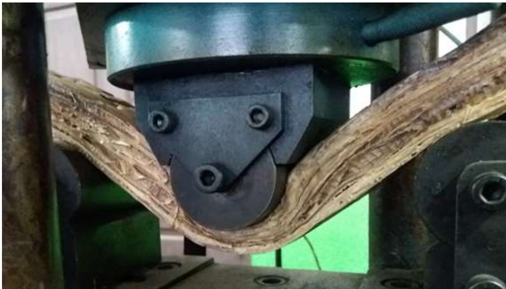
Figure 4. Flexural Test Conditions on Artificial Wood
