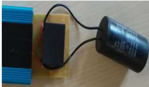
Figure 5. Capacitors in Energy Storage Devices
