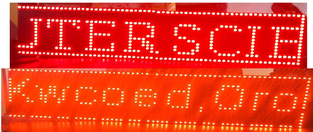
Figure 9. Display Text with Spacing between Character (One Column of) and a Complete off Module between Nine Words
