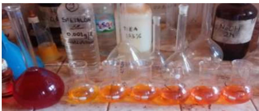
Photo 1. Helianthine stock and daughter solutions for the calibration curve.
