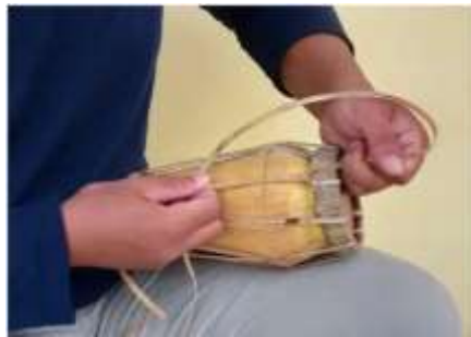
Figure 9. Follower Installation Process of Drum Binge
